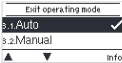
In the menu "4. Operating mode" the controller can either be placed in automatic mode, switched off or placed in a manual operating mode.
